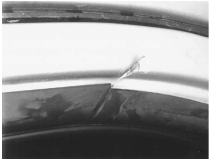
FIG. 4—Picture showing the impact found on the front upper part of the right front passenger door of the victim’s car.
